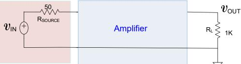
d) If two of these amplifiers are cascaded, they also form a two-port amplifier. Determine the amplifier parameters for the cascaded amplifiers.
